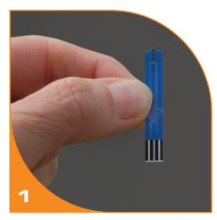
Remove sensor and place into analyser.
